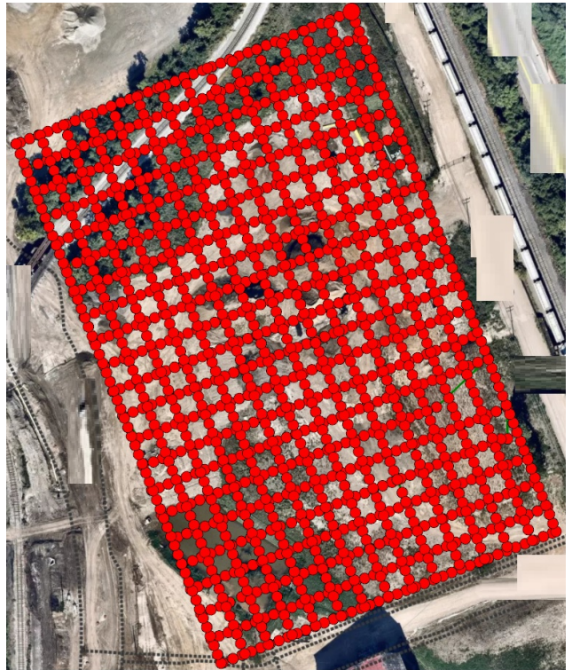
Figure 12. Data collection. We collect our poses for our Mill 19 dataset using a grid pattern as shown. Collecting footage across a 200,000\text{ m}^2 area takes approximately 2 hours.
