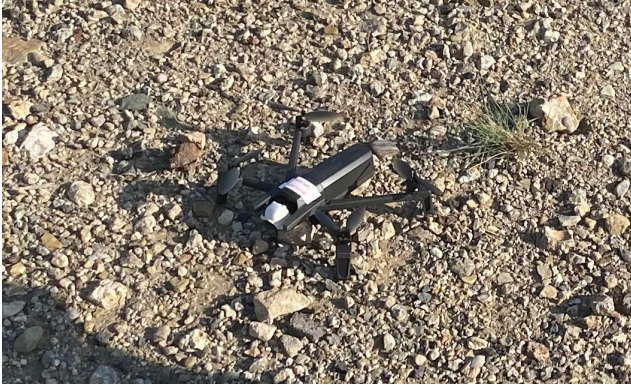
Figure 10. Parrot ANAFI drone. The drone used to collect data for the Mill 19 dataset. The drone comes equipped with a 4K Camera, GPS, and an inertial measurement unit (IMU) from which we derive initial camera poses.
